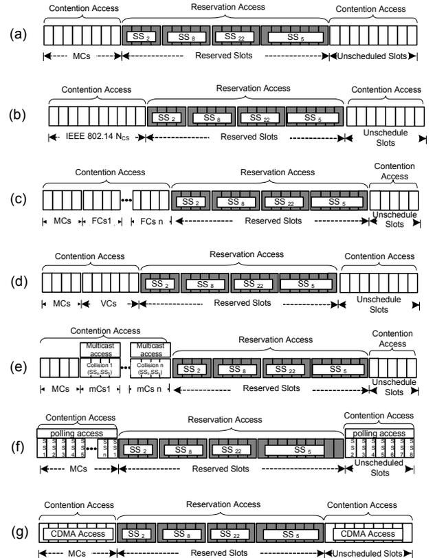
Fig. 2. Uplink frame structure of Contention Slot Allocators. (a) Simple-CSA, (b) IEEE 802.14 Variable-CSA, (c) Forced-CSA, (d) Variable-CSA, (e) Multicast-CSA, (f) Collision Free-CSA and (g) CDMA-CSA.
