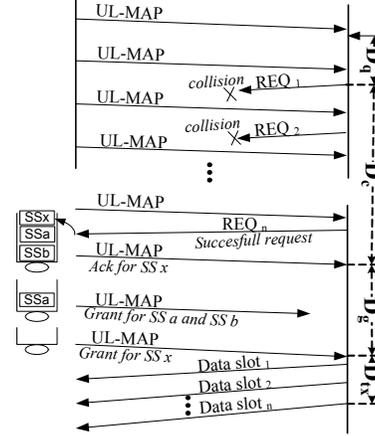
Fig. 3. Access delay components.
