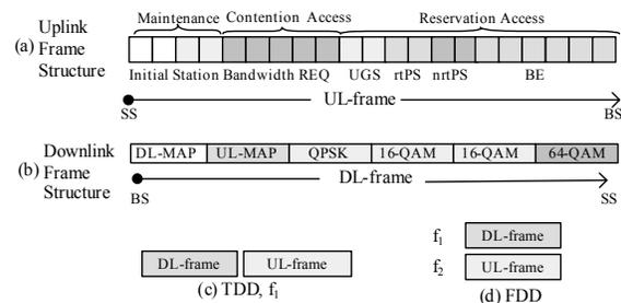
Fig. 1. Frame structure for TDD and FDD access.
